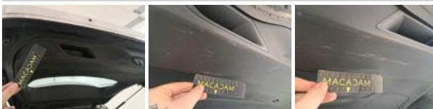
Boot lid covering R, Scratch(es), Smart repair
